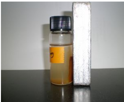
Fig: 3 Photograph showing super paramagnetic behaviour of PPy- \text{Fe}_3\text{O}_4 nanoparticles
